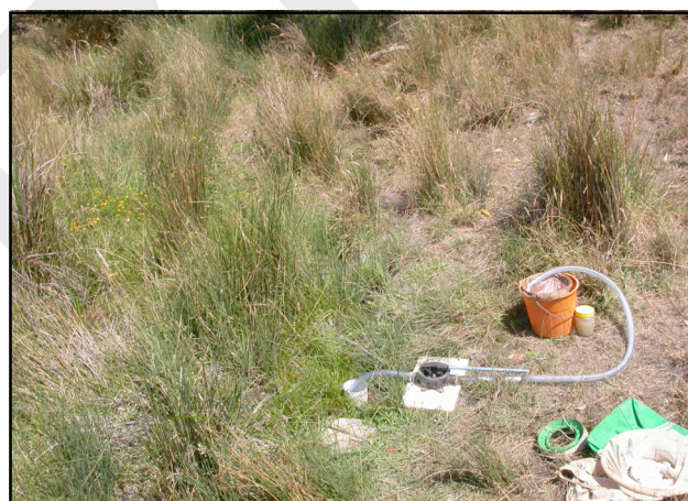
Figure 1. Schematic overview of a groundwater fed marshland fitted with a bore for collecting stygofauna. Figure 2. Bore with manual diaphragm pump.
