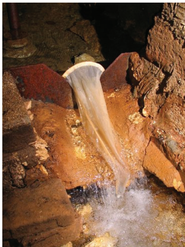
Fig. 6. Stygofauna net filtering the entire flow of the subterranean stream passing through the notched weir in Grants Well in 2006. Photo: Ross Anderson.
