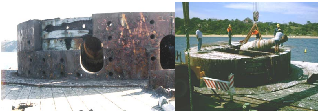
Figure 5: HMVS Cerberus with guns removed from one turret and being extracted from another 2004 © The Age
