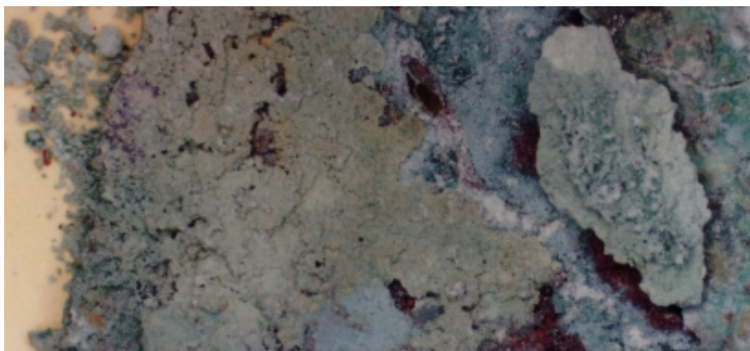
Figure 1. Amorphous bronze corrosion products from a cooking pot handle.
