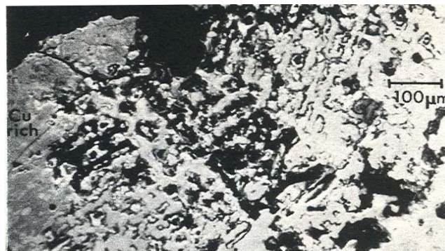
FIGURE 3 — A scanning electron micrograph of the seaward surface of a bronze pintle brace pin. The polished transverse section shows copper-rich areas as a medium gray while the tin and lead-rich phases are lighter in tone. The loss of the copper-rich phase close to the seawater interface is readily apparent. Full width is approximately 790 \mu\text{m} .
