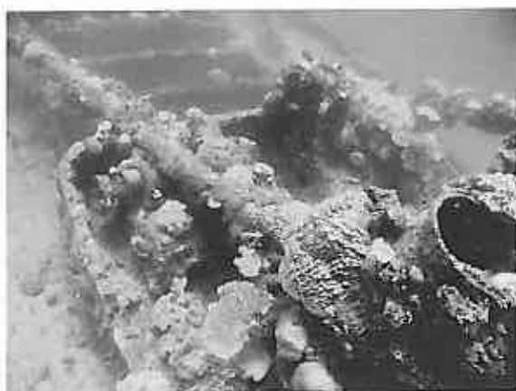
Figure 2. Extensive encrusting marine growth on the deck of the Fujikawa Maru with thicker growth surrounding the broken derrick. Photo Bill Jeffery.
